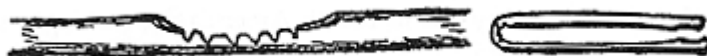
Notch the middle of the stick before bending it into fire tongs.
